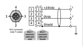
Note: Pump (BG45) needs:24 Vdc (min. 4A) Power supply
